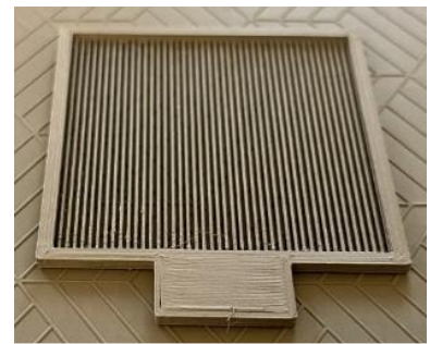
Fig. 1 Photograph of 3D printed polariser made of polyethylene terephthalate glycol (PETG) ferromagnetic composite.
