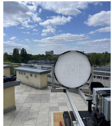
Fig. 1 Outdoor measurement setup for the longrange W-band
